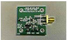
*Objective: To measure the phase noise of the 2.4GHz Monolithic Voltage Controlled Oscillator for use in 802.11b DSSS WLAN.*
